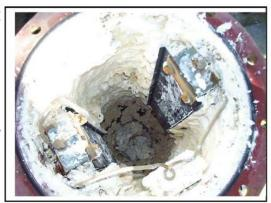
The scale formation theory states that water in its natural state contains a variety of dissolved solids, including the main ones: Ca(HCO3)2 and Mg(HCO3)2.
